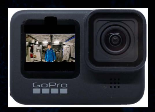
The camera of the Media Set is provided with a front screen that offers the possibility, for the crew, to see, in real time, what is the actual field of view of the camera and how he/she appears in the video.
